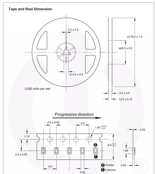
Note: Tolerances are ±0.1mm unless otherwise stated. All dimensions in mm.
