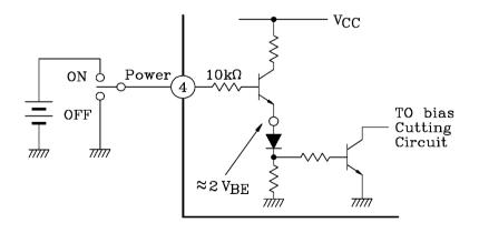
(Fig.-3) With (4) Pin set to High, Power is turned ON.
