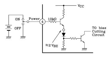
Fig.3 With 4 Pin set to High, Power is turned ON.
