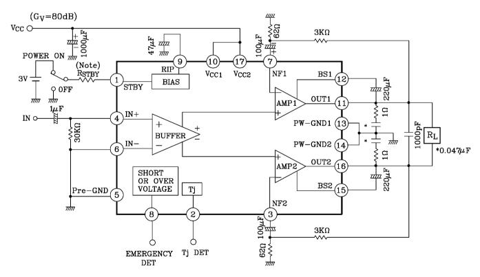
(Note) The purpose of  $R_{\,\rm STBY}$  is current limiting resistance.
