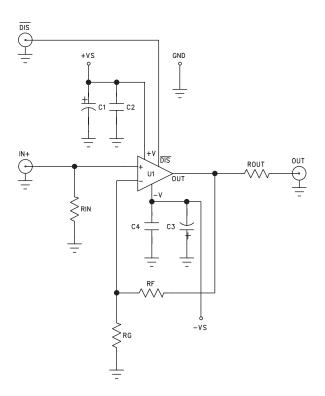
Figure 6: Evaluation Board Schematic (SOIC pinout shown)
