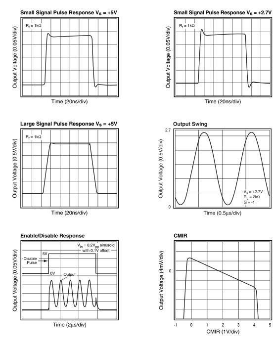
The KM4100/KM4101 are single supply, general purpose, voltage-feedback amplifiers fabricated on a complementary bipolar process using a patent pending topology. They feature a rail-to-rail output stage and are unity gain stable. Both gain bandwidth and slew rate are insensitive to temperature.
