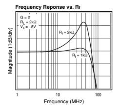
Figure 2: Frequency Response vs. R<sub>f</sub>
