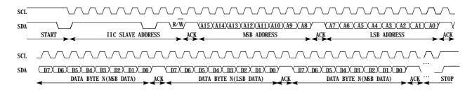
Figure 4. SDA line and SCL line (Write Operation)
