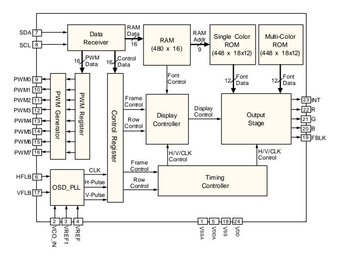
Figure 1. Functional Block Diagram of KS2501
