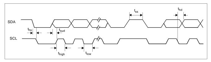
Figure 3. <sup>2</sup>C Bus Timing Diagram
