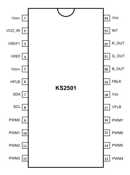
Figure 2. Pin Configurations
