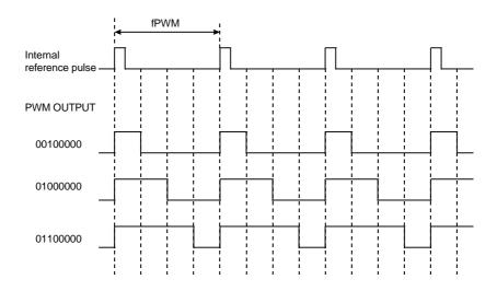
The frequency of PWM signal (fPWM) is dependent on the horizontal flyback signal frequency and horizontal mode (320dots/line, ...) as shown in the following table.
