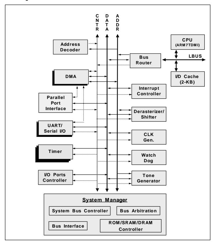
Figure 1. KS32C6200 Block Diagram
