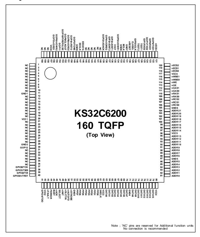
FIGURE 2. KS32C6200 PIN ASSIGNMENTS
