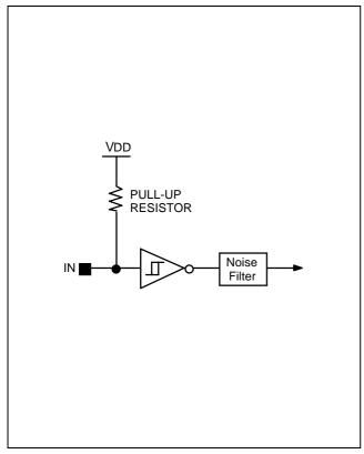
**Figure 1-4. Pin Circuit Type A (RESET)**
