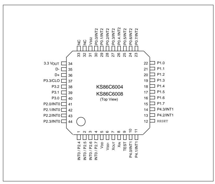
Figure 1-3. Pin Assignment Diagram (44-Pin QFP Package)
