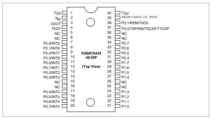
Figure 1-3. Pin Assignment (40-Pin DIP Package)
