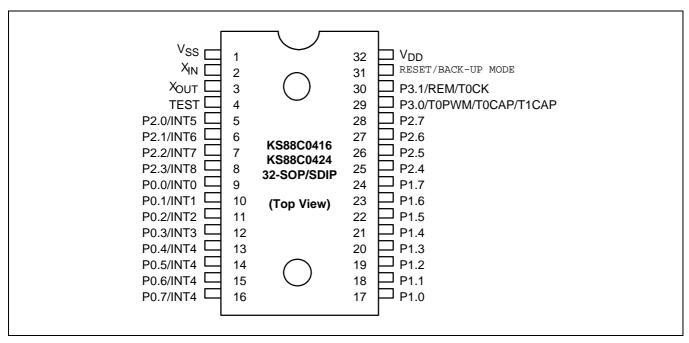
Figure 1-2. Pin Assignment (32-Pin SOP/SDIP Package)
