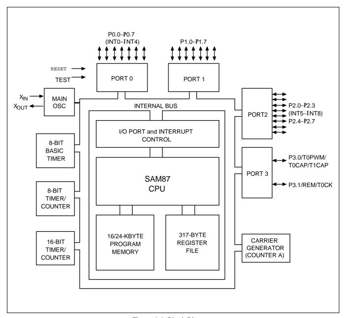
Figure 1-1. Block Diagram
