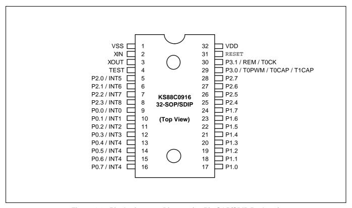
Figure 1-3. Pin Assignment Diagram (32-Pin SOP/SDIP Package)
