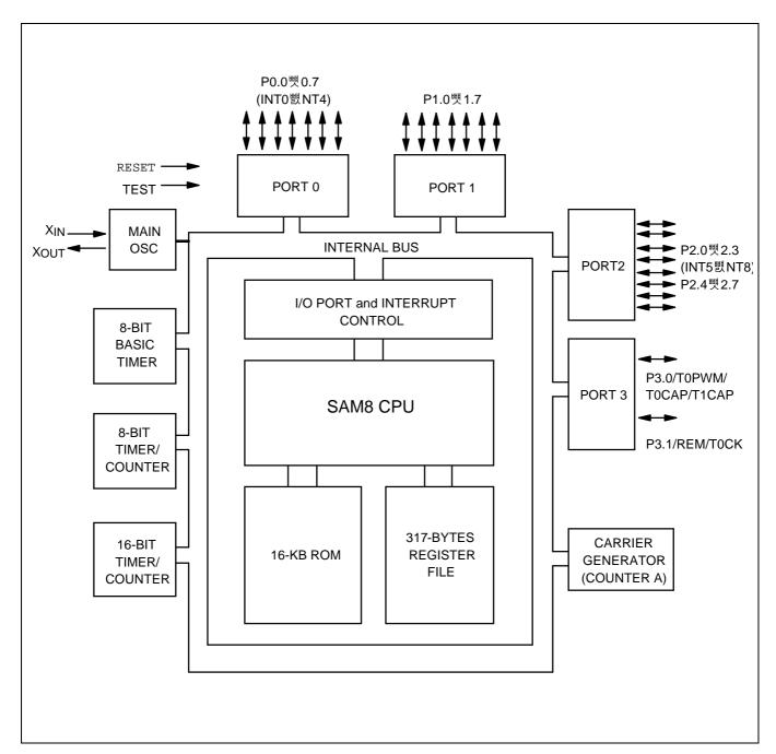
Figure 1-2. Block Diagram
