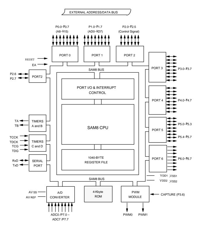
NOTE: KS88C4404 has a 4-Kbyte internal program memory, but KS88C4400 has no internal program memory.
