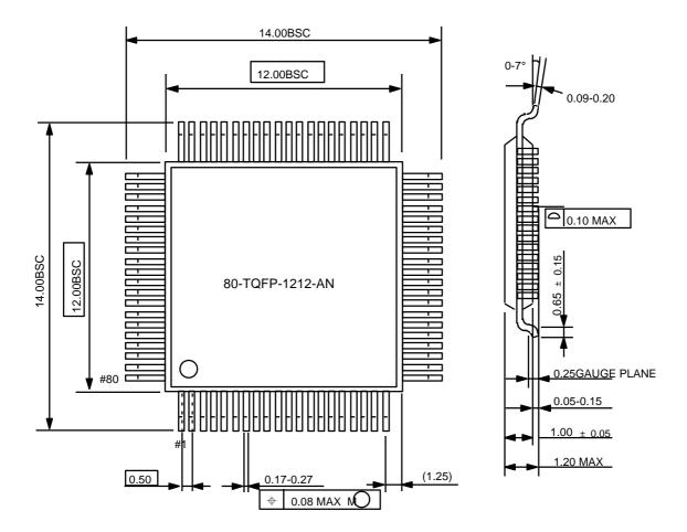
**NOTE** : Dimensions are in millimeters.
