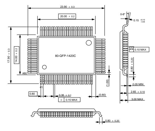
$\ensuremath{\textbf{NOTE}}$  : Dimensions are in millimeters.
