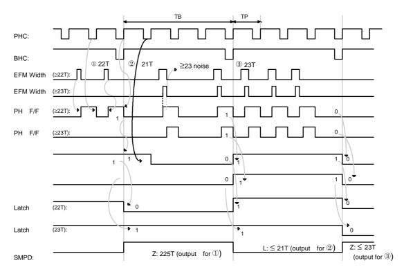
Fig. 18 The timing chart of SMSD output when gain is 'H'
