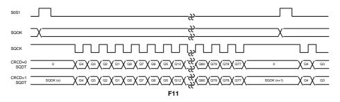
Comment: If the SQOK of the subcode Q data is "H", subcode data is outputted to SQDT according to subcode, and it is "L" is outputted.
