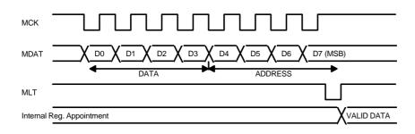
Fig. 3 mCOM DATA INPUT TIMING CHART
