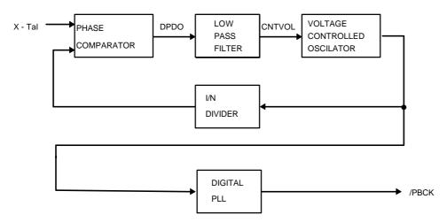
Fig. 21: The application diagram of Digital PLL
