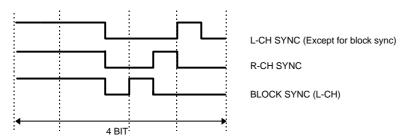
Fig 15. Preamble signal
