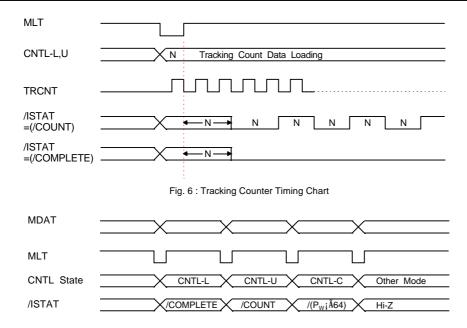
Fig 7. /ISTAT output signal according to CNTRL Register
