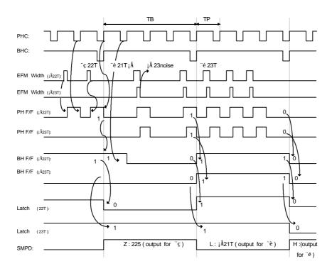
FIG.20 : Timing chart of SMPD output when the gain is "H" in the speed mode
