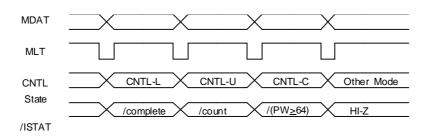
Fig.3. /ISTAT output signal according to CNTL Register
