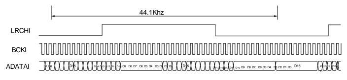
Fig.21. Timing chart of signal ESP IC outputting to DSP
