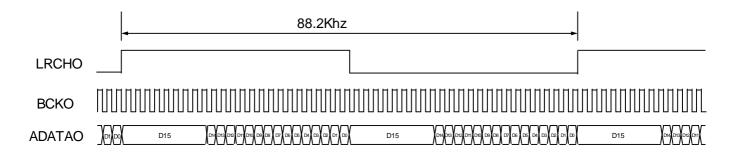
Fig.20. Timing chart of signal outputting to ESP IC
