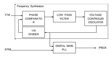
Fig.17. Digital PLL circuit diagram
