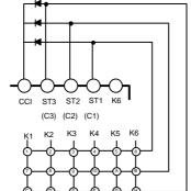
\* Custom code bit consists of 3 bits (C1,C2,C3), and makes 8 custom codes.
