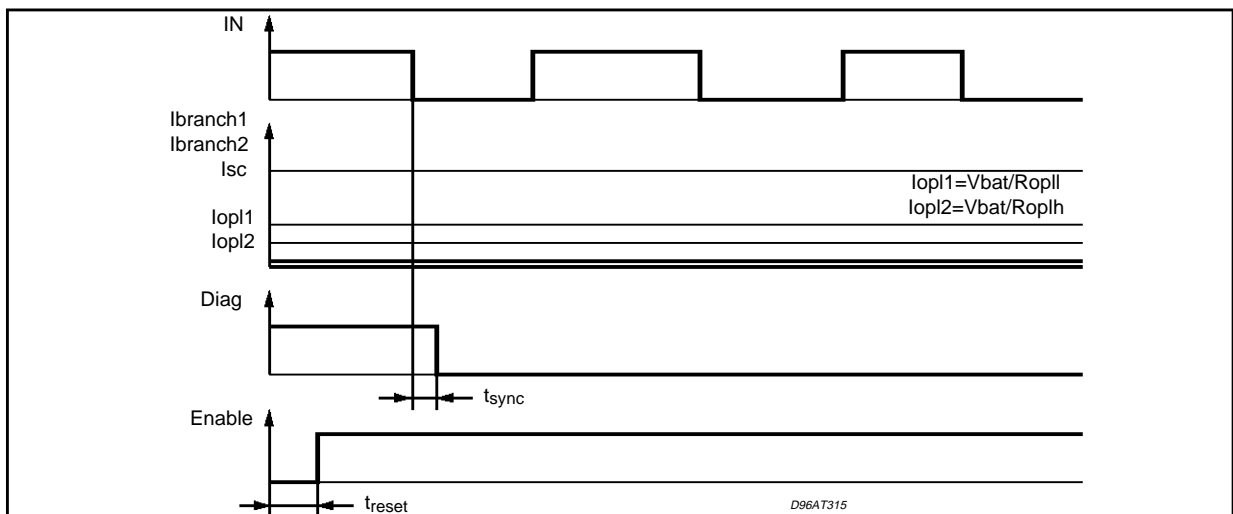
Figure 10: Open Load Condition 2: No Current after \overline{ENABLE}
