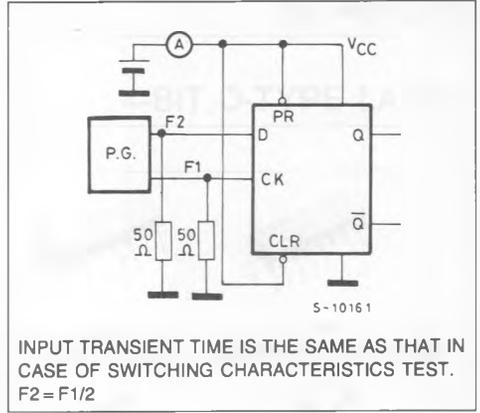
INPUT TRANSIENT TIME IS THE SAME AS THAT IN CASE OF SWITCHING CHARACTERISTICS TEST.  $F2 = F1/2$
