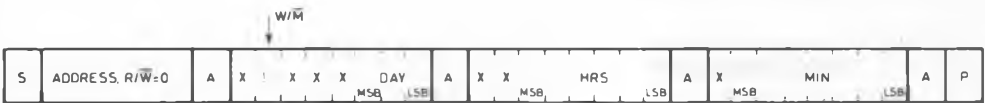
Fig. 3b - Data format for one cycle address/write (with day of week indication)
