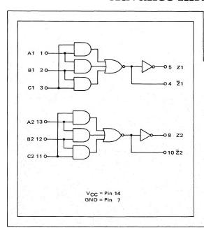
This integrated circuit offers the designer additional versatility in logic design. When any two or all three of the inputs are raised to the "1" level, the output goes to the "1" level. The output, Z, and its complement,  $\overline{Z}$ , are both available.
