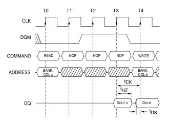
NOTE: A CAS latency of three is used for illustration. The READ command may be to either bank, and the WRITE command may be to either bank. If a CAS latency of one is used, then DQM is not required.
