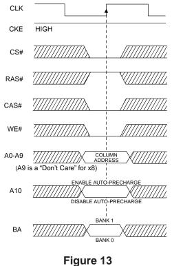
Figure 13 WRITE COMMAND provided coincident with the new command applies to the new command. An example is shown in Figure 15. Data n + 1 is either the last of a burst of two or the last desired of a longer burst. The Micron 16Mb SDRAM uses a pipelined architecture and therefore does not require the 2n rule associated with a prefetch architecture. A WRITE command can be initiated on any clock cycle following a previ-
