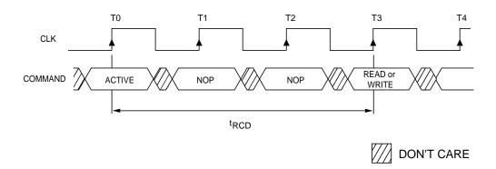
Figure 4 EXAMPLE: MEETING <sup>t</sup>RCD (MIN) WHEN 2 < <sup>t</sup>RCD (MIN)/<sup>t</sup>CK < 3
