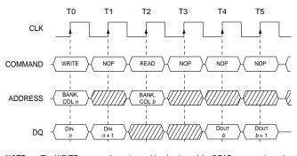
**NOTE:** The WRITE command may be to either bank, and the READ command may be to either bank. DQM is LOW. CAS latency = 2 for illustration.
