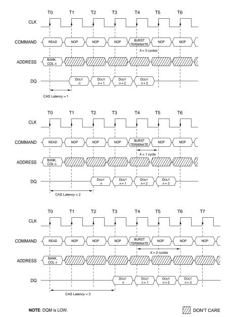
Figure 12 TERMINATING A READ BURST
