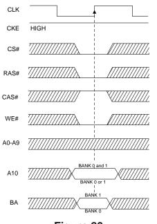
Figure 20 PRECHARGE COMMAND be the input data applied one clock previous to the BURST TERMINATE command. This is shown in Figure 19, where data n is the last desired data element of a longer burst.
