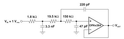
Figure 29. OPAx364 Configured as 3-Pole, 20-kHz, Sallen-Key Filter
