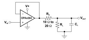
Figure 22. Improving Capacitive Load Drive
