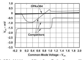
Figure 20. OPAx364 Linear Offset Over Entire Common-Mode Range
