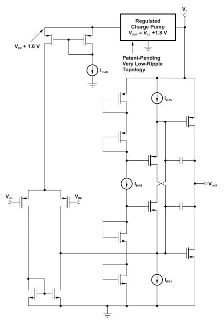
Figure 21. Simplified Schematic
