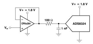
Figure 26. OPAx364 Directly Drives the ADS8324
