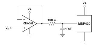
Figure 27. Driving the 12-Bit A/D Converter on the MSP430
