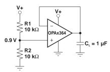
Figure 25. OPAx364 Provides a Stable Reference Voltage
