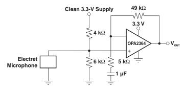
Figure 28. Microphone Preamplifier
