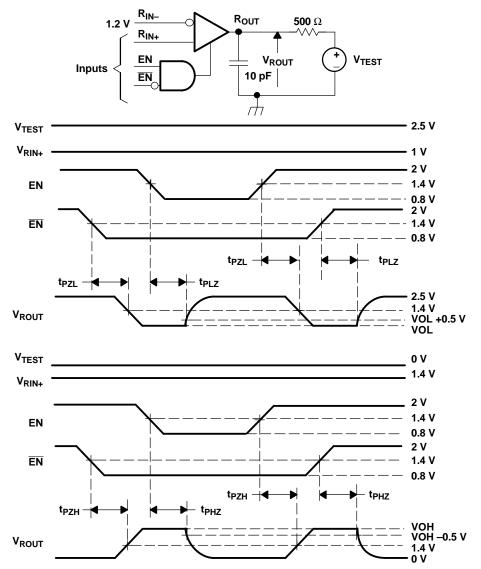
A. All input pulses are supplied by a generator having the following characteristics:  $t_r$  or  $t_f \le 1$  ns, signaling rate = 500 kHz, duty cycle = 50 ±2%, C<sub>L</sub> includes instrumentation and fixture capacitance within 0,06 mm of the D.U.T and is ±20%.
