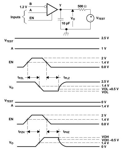
A. All input pulses are supplied by a generator having the following characteristics:  $t_r$  or  $t_f \le 1$  ns, signaling rate = 500 kHz, duty cycle = 50 ±2 %,  $C_L$  includes instrumentation and fixture capacitance within 0,06 mm of the D.U.T and is ±20%.
