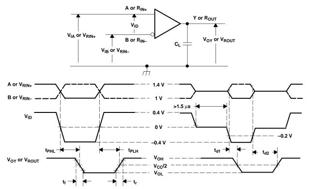
A. All input pulses are supplied by a generator having the following characteristics:  $t_r$  or  $t_f \le 1$  ns, signaling rate = 250 kHz, duty cycle = 50 ±2%, C<sub>L</sub> includes instrumentation and fixture capacitance within 0,06 mm of the D.U.T and is ±20%.
