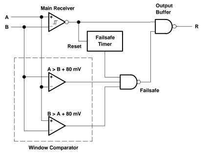
Figure 16. Receiver With Active Failsafe
