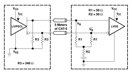
Figure 17. LVPECL or PECL to Remote Wide Common-Mode LVDS Receiver
