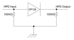
Figure 1. HPD Test Circuit
