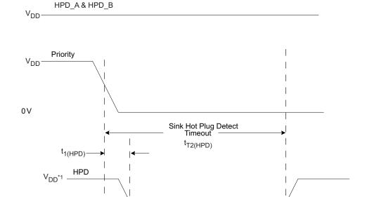
Figure 3. HPD Timing Diagram #2
