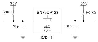
Figure 6. Auxiliary Channel Test Circuit (CAD = HIGH)
