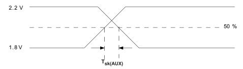
Figure 7. Auxiliary Channel Skew Measurement
