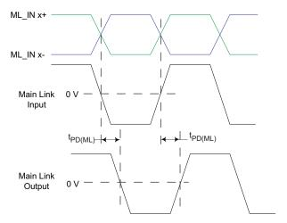
Figure 12. Main Link Delay Measurements
