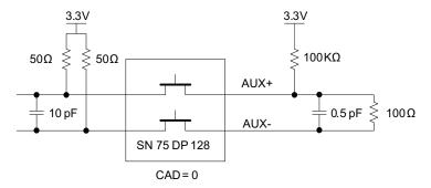
Figure 5. Auxiliary Channel Test Circuit (CAD = LOW)
