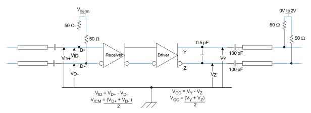
Figure 10. Main Link Test Circuit
