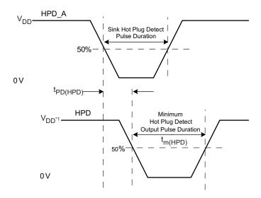
Figure 2. HPD Timing Diagram #1
