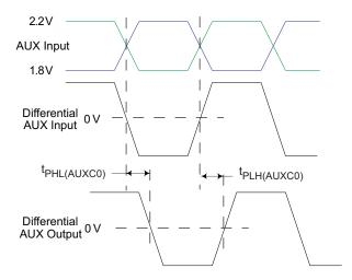
Figure 8. Auxiliary Channel Delay Measurement (CAD = LOW)
