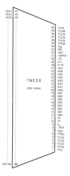
Note: The above diagram shows the pin configuration of the LSI chip; it does not show the configuration of the tape carrier package.
