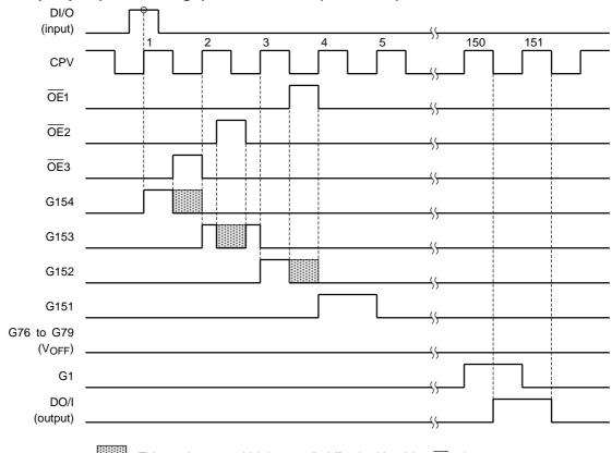
: This part is output which is controlled (fixed to V\_OFF) by  $\overline{\mbox{OE}}$  pin.
