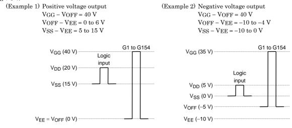
Note: The logic input here means input pins DI/O, DO/I, CPV, MODE and  $\overline{OE1}$  to  $\overline{OE3}$ . The amplitude between V<sub>SS</sub> and V<sub>DD</sub> is applied to above pins. Make sure that the voltage applied to the U/D pin is a high (= V<sub>DD</sub>) or low (= V<sub>SS</sub> or V<sub>EE</sub>) DC-level voltage.
