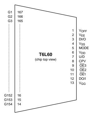
The above diagram shows the device's pin configuration only and does not necessarily correspond to the pad layout on the chip. Please contact Toshiba or our distributors for the latest TCP specification.
