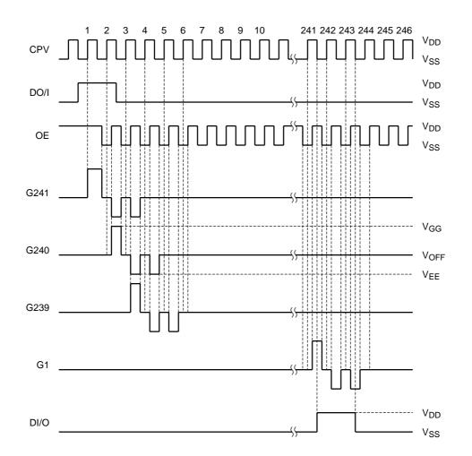
• 2CPV input drive (D/U = High level, MODE = Low level)
