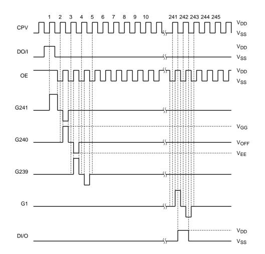
• 1CPV input drive (D/U = High level, MODE = Low level)
