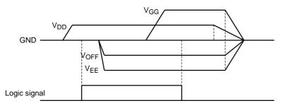
\*Logic signal includes High and Low levels (DC voltage) as well as signal rise and fall.
