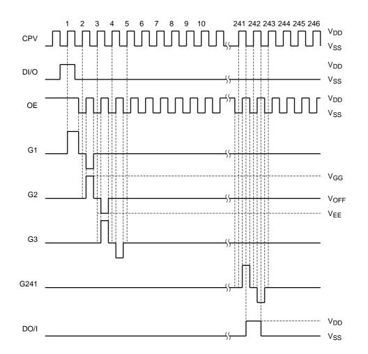
• 1CPV input drive (D/U = Low level, MODE = High level)
