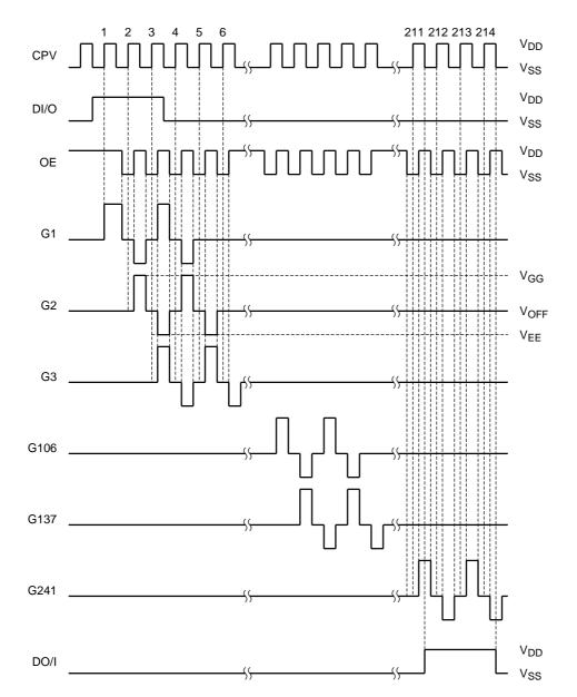
• 3CPV input driver (D/U = Low level, MODE = High level)
