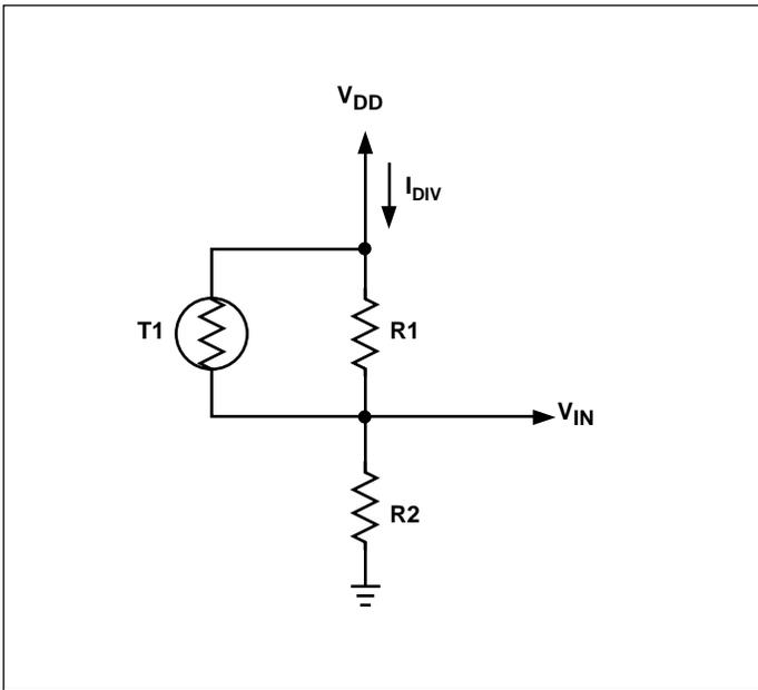
Figure 5. Temperature Sensing Circuit
