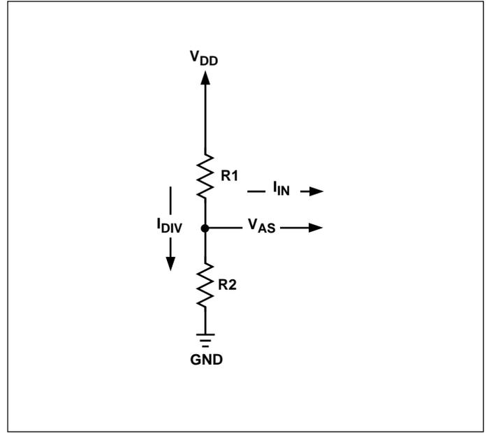
Figure 6.  $V_{AS}$  Circuit
