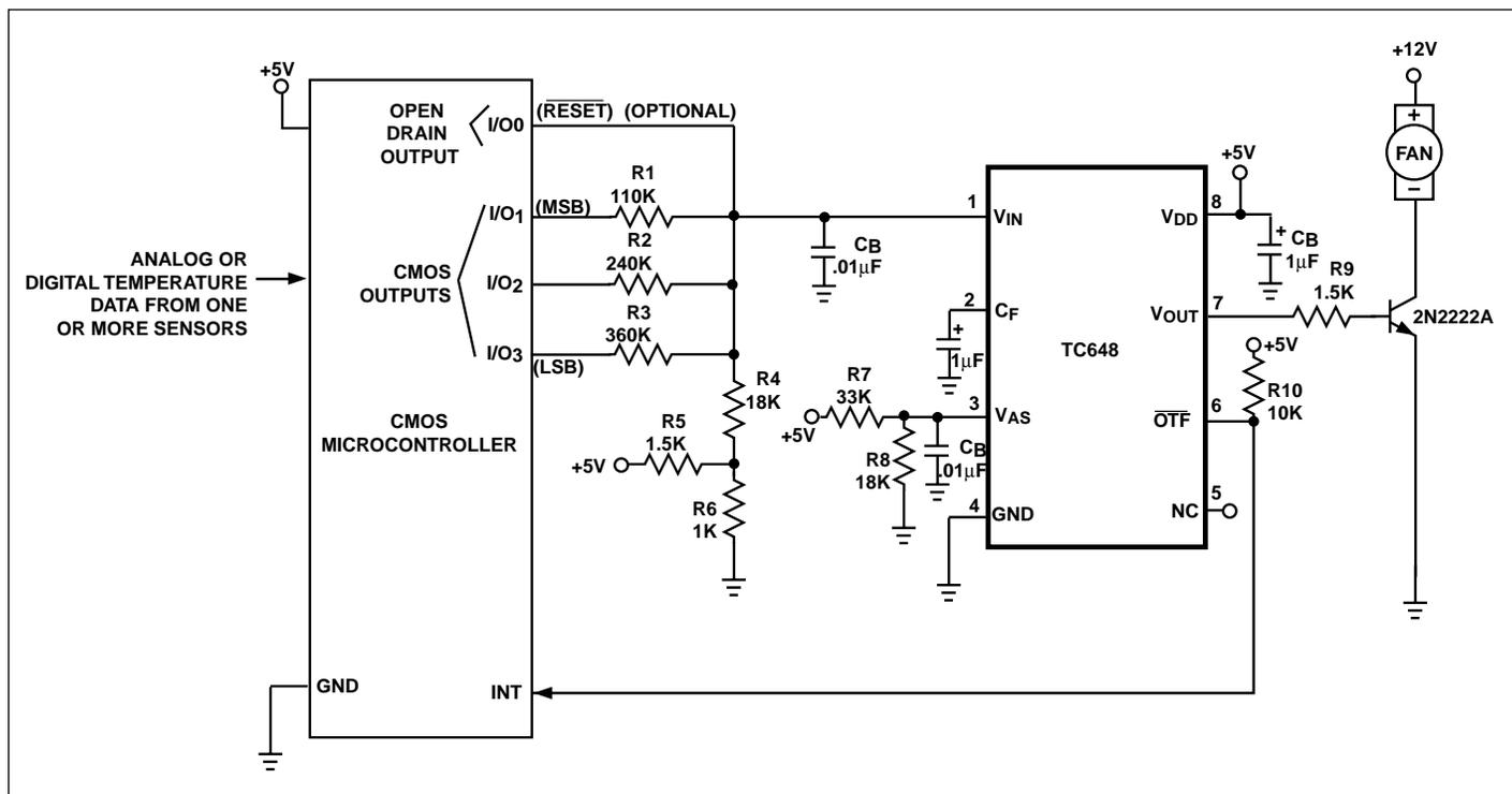
Figure 11. TC648 as a Microcontroller Peripheral
