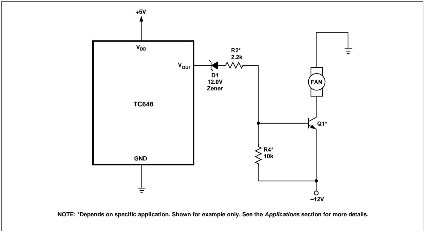
Figure 8. Powering the Fan from a Negative Supply
