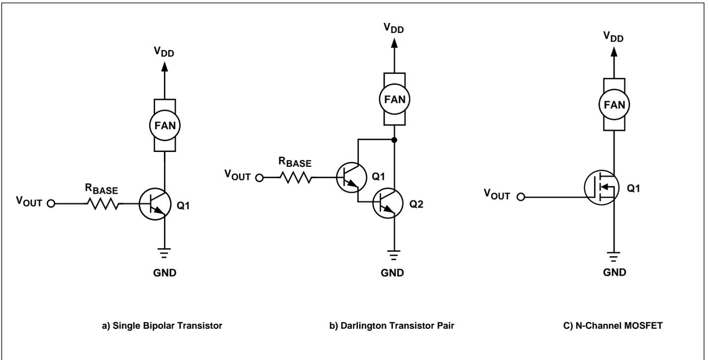
Figure 7. Output Drive Transistor Circuit Topologies
