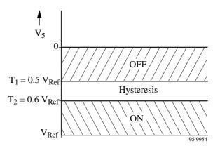
Figure 7. Trigger condition, Pin 5
