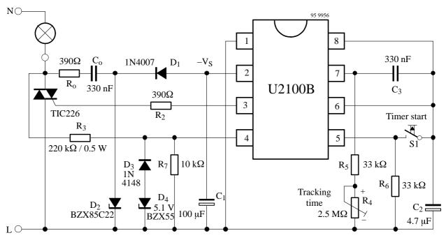
Figure 9. Lamp time control 18 sec. to 23 min. for two wire systems
