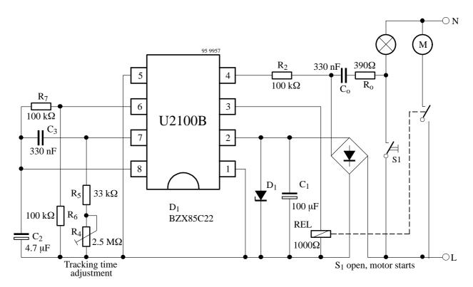
Figure 10. Fan tracking time control 18 sec. to 23 min.
