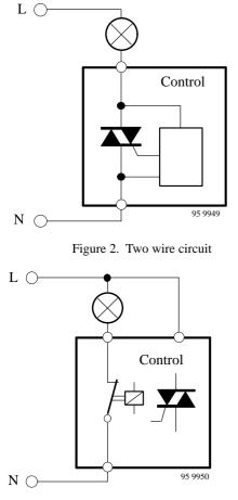
Figure 3. Three wire circuit
