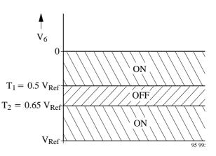
Figure 8. Trigger condition, Pin 6
