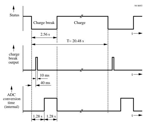
Figure 6. Operating sequence of voltage measurements
