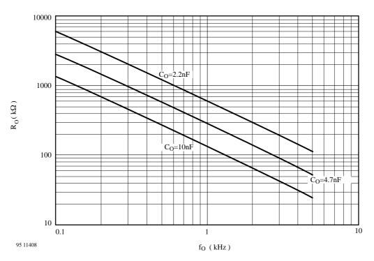
Figure 9. Frequency versus resistance for different capacitance values
