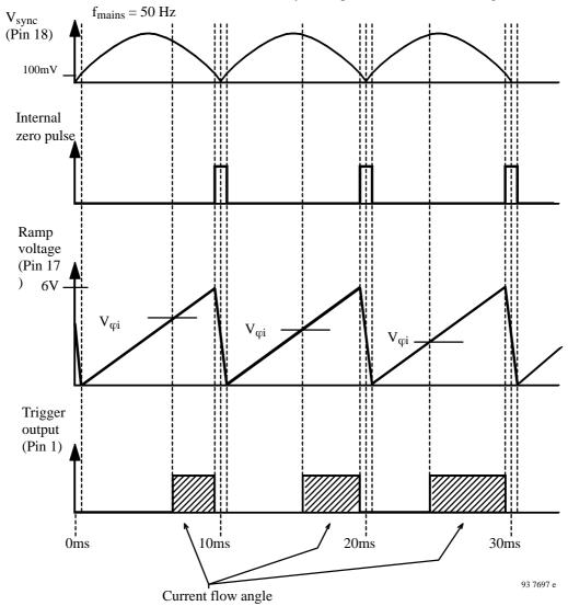
Figure 8. Phase control function diagram
