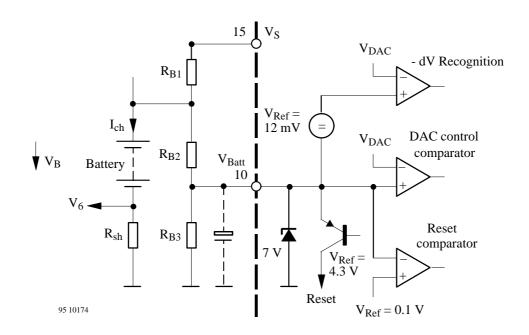
Figure 5. Input configuration for the battery voltage measurement
