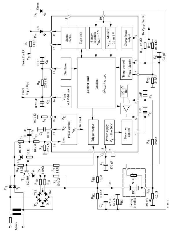
Figure 2. Block diagram with external circuit (DIP pinning)
