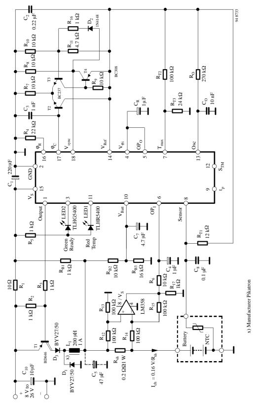
Figure 10. Car battery supplied charge system with high side current detection for four NiCd/NiMH cells @ 800 mA
