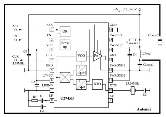
Figure 5. Application circuit
