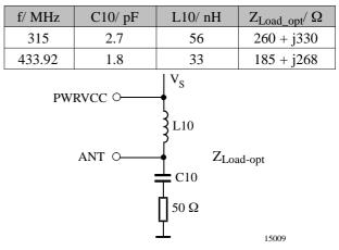
Figure 4. Measurement output network
