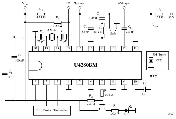
Figure 7. Application circuit
