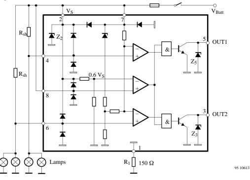
Figure 1. Schematic and application circuit
