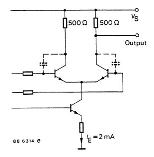
Figure 4. ECL output circuit
