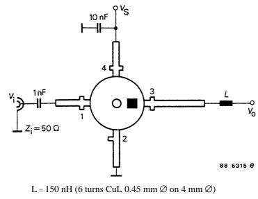
Figure 2. Test circuit
