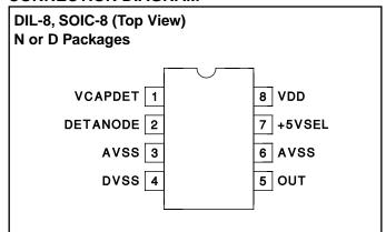
**ELECTRICAL CHARACTERISTICS** Unless otherwise specified,  $3.0V \le VDD \le 3.5V$  and +5VSEL = GND, or  $4.5V \le VDD \le 5.5V$  and +5VSEL = VDD, CDETECTOR < 56pF, CLOAD = 40pF,  $0^{\circ}C < TA < 70^{\circ}C$ , TA = TJ.
