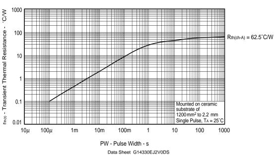
TRANSIENT THERMAL RESISTANCE vs. PULSE WIDTH
