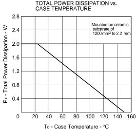
**Remark** Mounted on ceramic substrate of 1200  $\text{mm}^2 \times 2.2 \text{ mm}$
