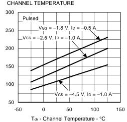
DRAIN TO SOURCE ON-STATE RESISTANCE vs.
