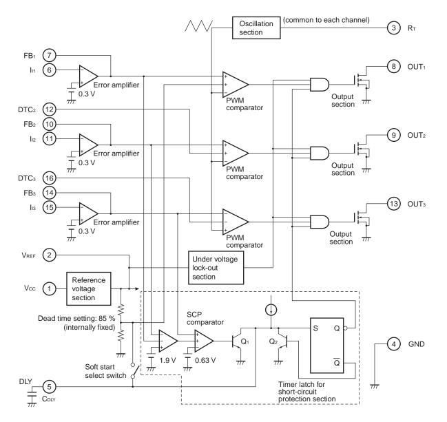
Figure 2-1 Block Diagram
