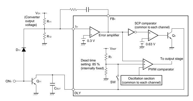
Figure 3-3 ON/OFF Control (channel 1 for step-up)
