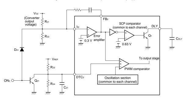
Figure 3-4 ON/OFF Control (channel 2: step-up)
