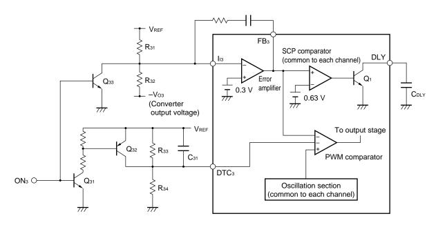
Figure 3-5 ON/OFF Control (channel 3: for inverted output)
