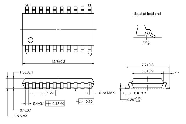
**NOTE** Each lead centerline is located within 0.12 mm of its true position (T.P.) at maximum material condition.
