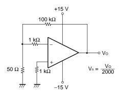
Figure 2 Channel Separation Measurement Circuit
