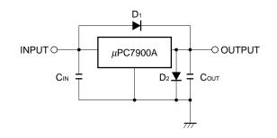
$\text{C}_{\text{IN}}$  : More than 2.2  $\mu\text{F}$
