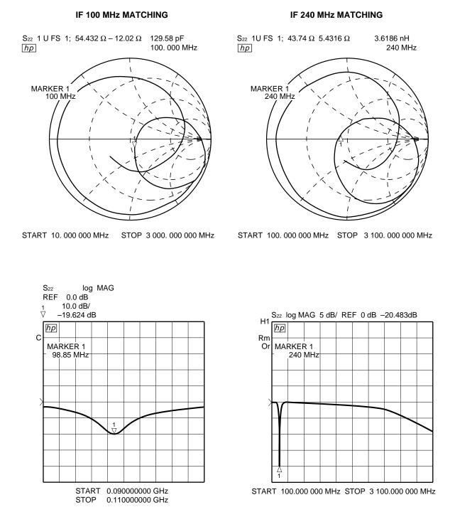
The data in this page are to make clear the test condition of impedance matched to next stage, not specify the recommended condition. The S<sub>22</sub> smith charts of the test fixture setting IC are normalized to Zo = 50  $\Omega$ , because the IC's load is the measurement equipment of 50  $\Omega$  impedance.
