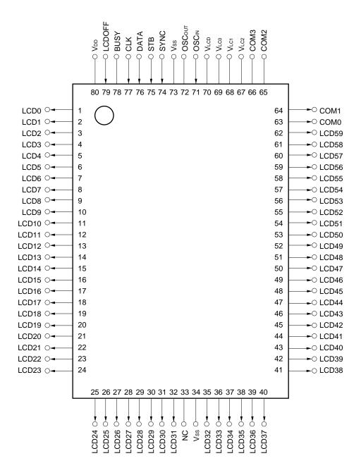
**Remark** Be sure to leave Pin 33 open since it is connected to the lead frame.
