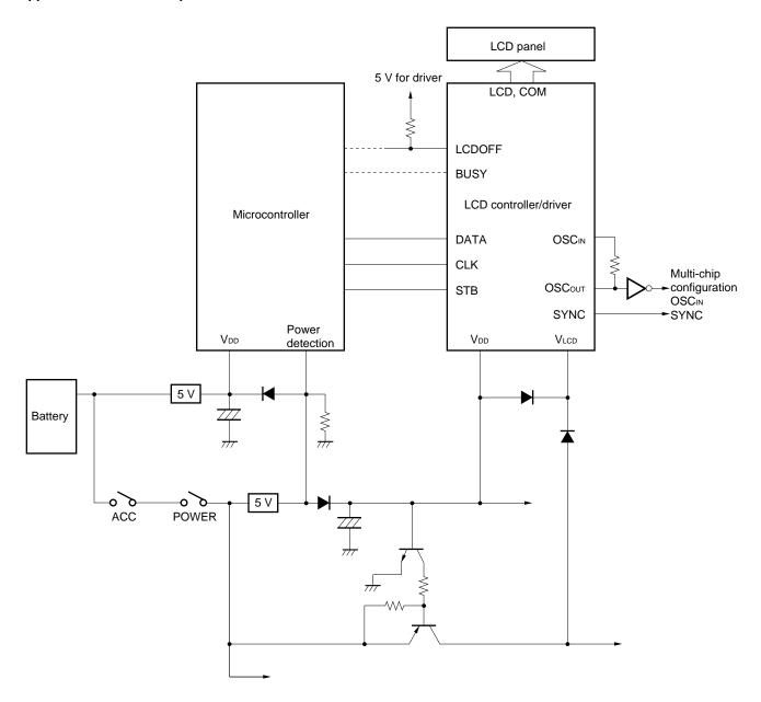
**Remark** Use low-V<sub>F</sub> diodes such as Schottky-barrier diodes, and make sure that V<sub>DD</sub>, V<sub>LCD</sub>, V<sub>I</sub>, etc. do not exceed absolute maximum ratings of the diodes.
