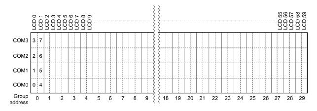
**Remark** During auto incrementing, incrementing past the last group address of each duty (for example group address 14 in the case of 1/2 duty) brings the counter back to "0."
