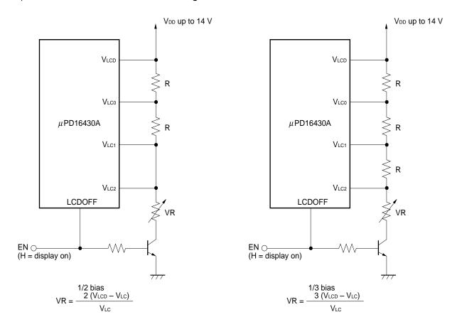
VLC is the peak value of the optimum drive voltage for LCD. (it varies depending on the LCD.)
