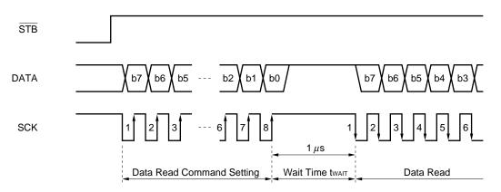
Caution As the DATA pin is an Nch open-drain output, a pull-up resistor must be connected externally (1 k $\Omega$  to 10 k $\Omega$ ).
