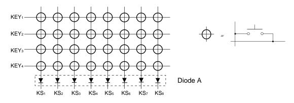
In this example, if 3 or more keys are simultaneously pressed, switches in the OFF state may be inadvertently judged as being ON.
