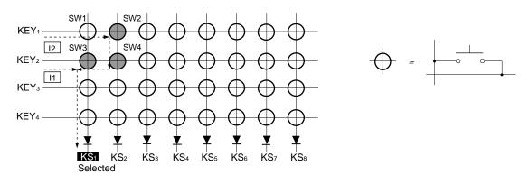
Also, if diode A is not connected, not only will the key data be unable to be read correctly, but the LCD may also be affected and the IC damaged or its characteristics degraded.
