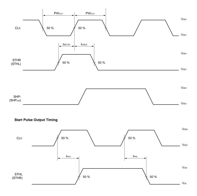
Remark The input/output timing of the start pulse is the same for simultaneous/successive sampling.
