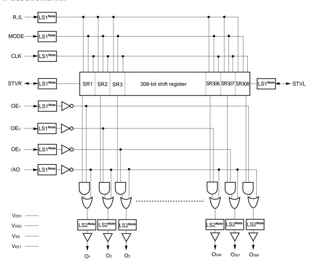
Note LS1: shifts CMOS level and internal level, LS2: shifts interval level and output level (VDD2 to VEE1).
