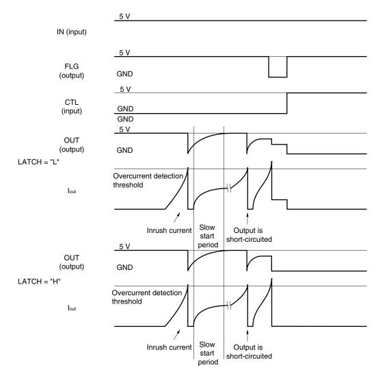
If an overcurrent is detected after the overcurrent detection delay time of 20  $\mu$ s, the IC executes a slow-start operation (output rise time: 5 ms TYP.) again.
