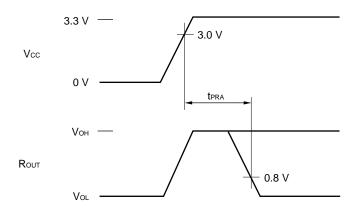
Receiver outputs are indefinite during reset release time (tPRA).
