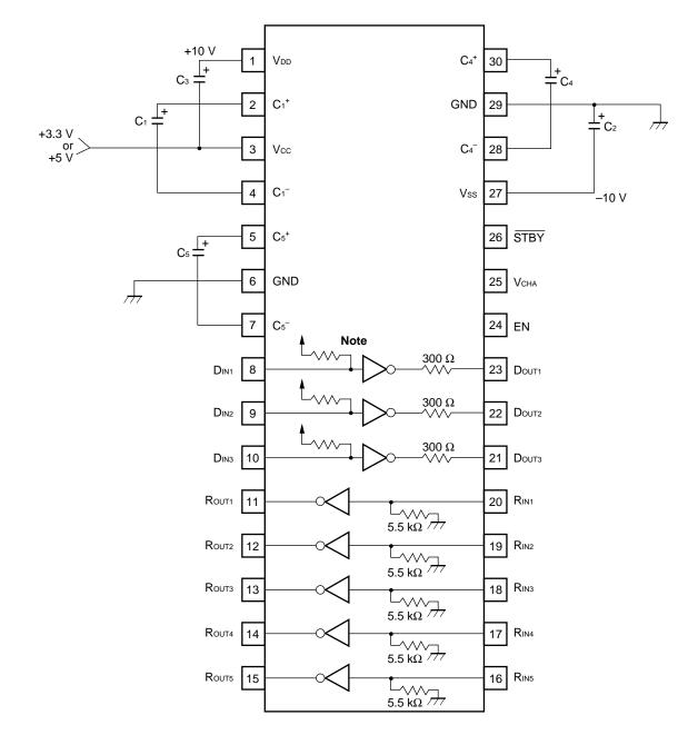
Note The pull-up resistors of the driver inputs are active resistors.
