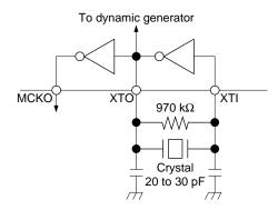
As in Figure 3-2, the clock can also be generated by supplying a system clock from outside to the XTI (No.4) pin. The system clock waveform at this time must satisfy the conditions in the electrical specifications (such as VIH, VIL under DC characteristics; and tMCK, tMWHM, tMWL under AC characteristics).
