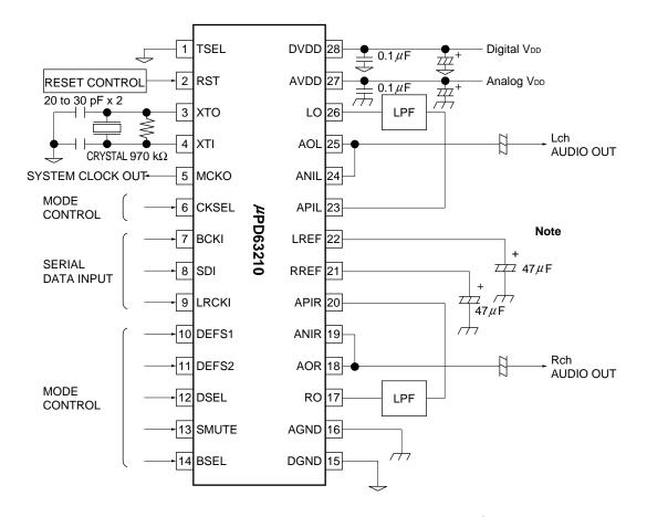
Figure 4-1. Application Circuit Example in Using Crystal Oscillation Circuits
