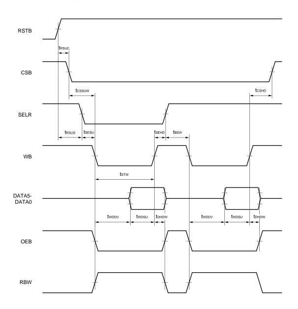
★ Parallel interface write timing 2 (when there are continual write cycles while CSB is low)
