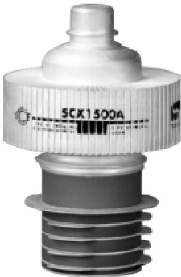
**T** The Svetlana 5CX1500A is a high-performance ceramic/metal power pentode designed for use as a highly linear Class AB1 linear amplifier. It may also be used as a high-gain Class C amplifier in HF radio frequency industrial processing applications such as plasma generation, sputtering and semiconductor manufacturing. The 5CX1500A filament is precision fabricated in a cylindrical mesh configuration for exceptional mechanical stability and long life.
